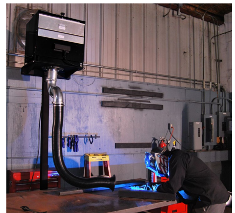
Model 400/450 Mounted Sentry frees up valuable benchtop space with fume extractor stand.
